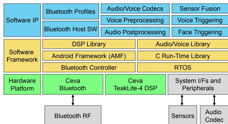
**Figure 1. Ceva's platform for wearable devices.** The company licenses this combination of its DSP IP, Bluetooth core, and software stack, enabling SoC designers to more easily develop custom solutions for wearables.
