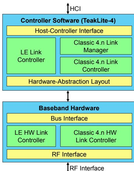
**Figure 2. Ceva Bluetooth implementation.** The MAC layer runs on the TeakLite-4 DSP, leaving only a small amount of hardware for the baseband.
