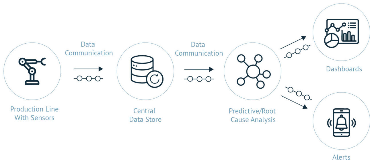
Predictive maintenance architecture enabled by edge AI (Image Credit: Copernilabs) [vi]
