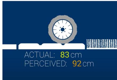
*Figure 2-3 Different surfaces can change the effective wheel circumference*
