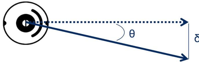
Figure 2-4 Angular error ( $\theta$ ) and corresponding positional error ( $\delta$ )
