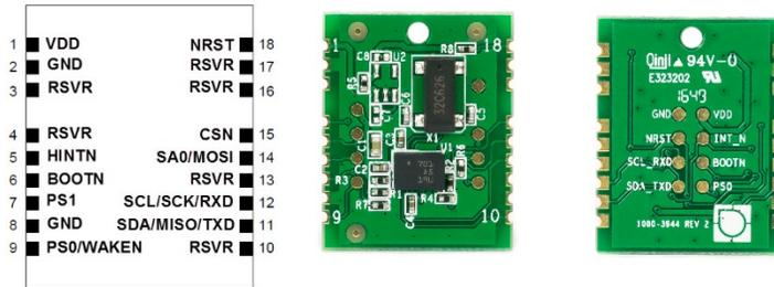
Figure 2: FSM30X Pinout
