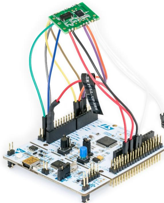
Figure 3: FSM30X connected to STM32F411RE Nucleo Board (I2C mode shown)
