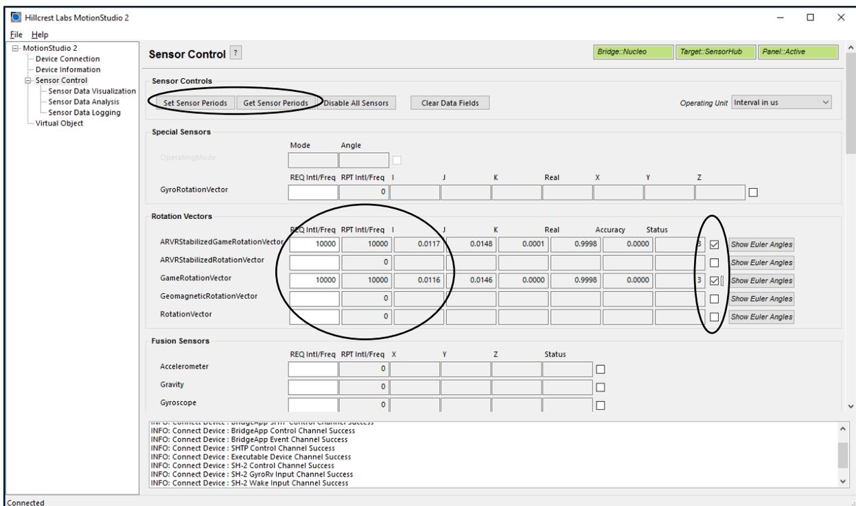
Figure 10: Sensor Control Panel in Freespace® MotionStudio 2
