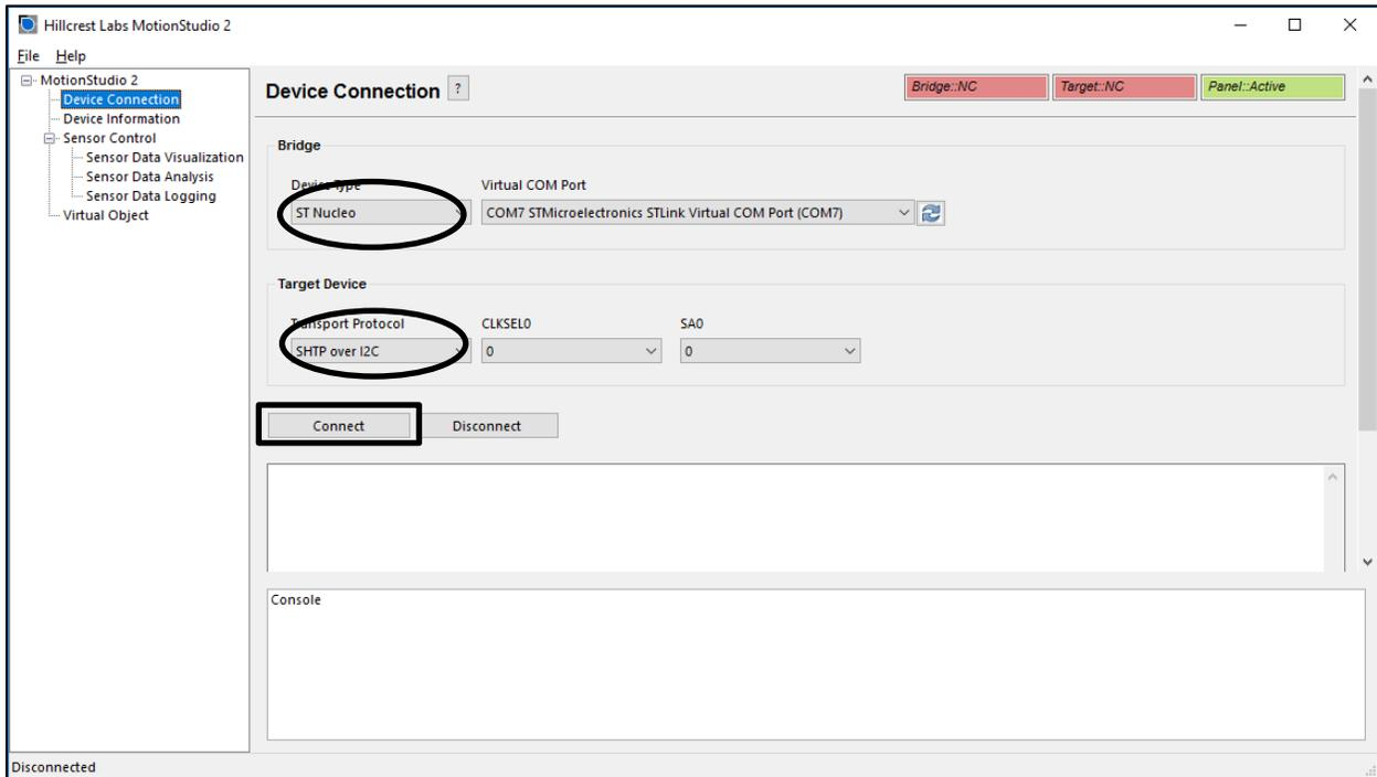
Figure 8: Device Connection Panel in Freespace® MotionStudio 2
