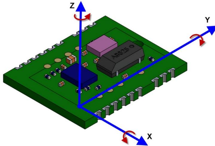
Figure 12: FSM30X Orientation
